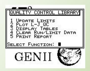
The GENESYS Genii Series multi-well gamma counter comes equipped with software to allow quality control evaluation and storage.
