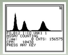
I125 and Co57 are counted simultaneously; spilldown is automatically subtracted.
